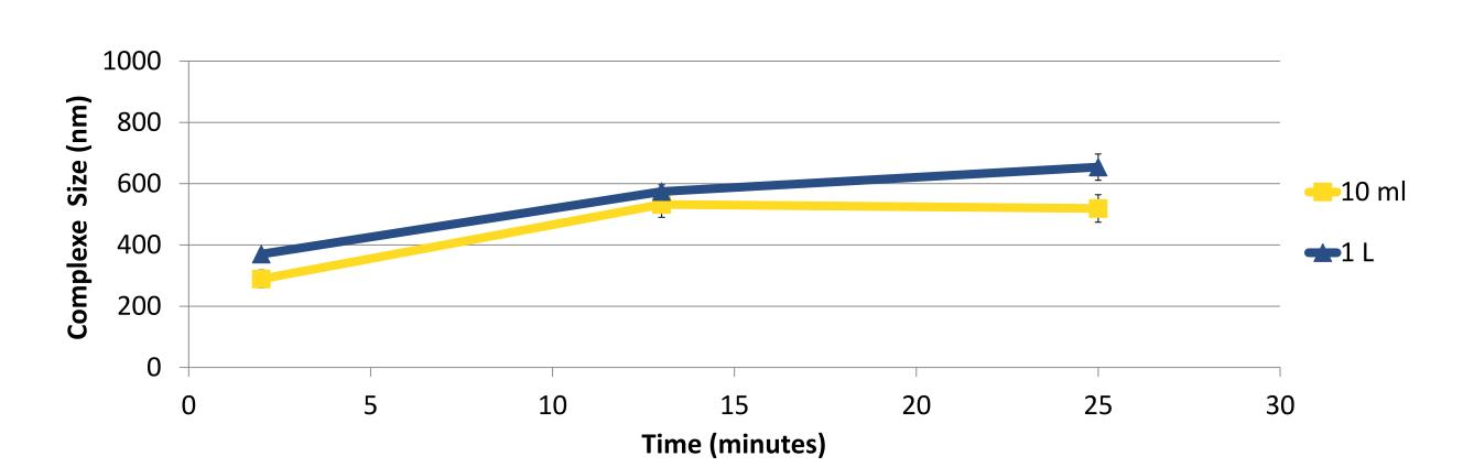
**DNA-PElpro® complex size is identical, independently from the volume of transfection mix preparation**. Complexes were prepared with a DNA concentration of 0.01 mg/mL of complex volume at a DNA:Reagent ratio of 1:4, either in 10 mL or 1 L. The size of the complexes was then measured at different time susing the Zetasizer Nanometer ZS (Malvern Instrument, Malvern, UK).
