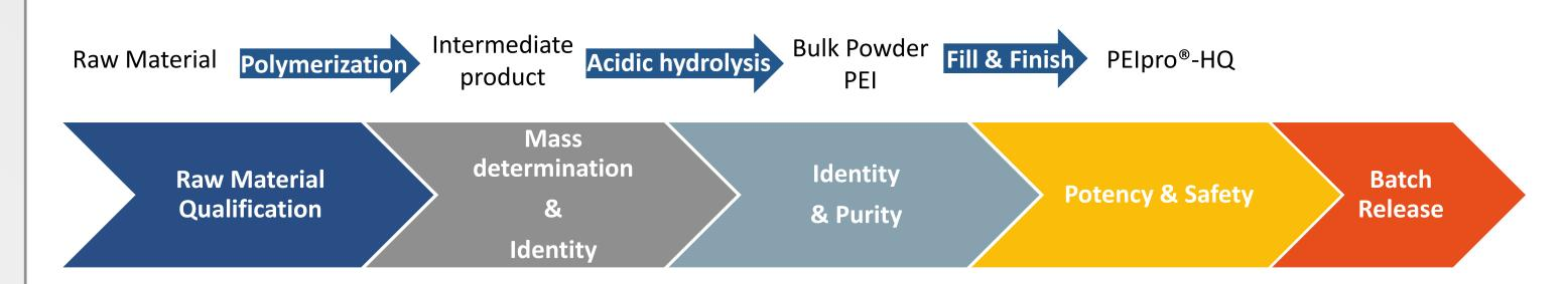
**Manufacturing process of PElpro® and PElpro®-HQ reagents**. The linear structure of PElpro® and the manufacturing process developed by Polyplus-transfection® ensure a high, stable and reproducible amount of protonable amines available for transfection while providing a fully deacylated molecule and an extremely low polymer chain length variation.
