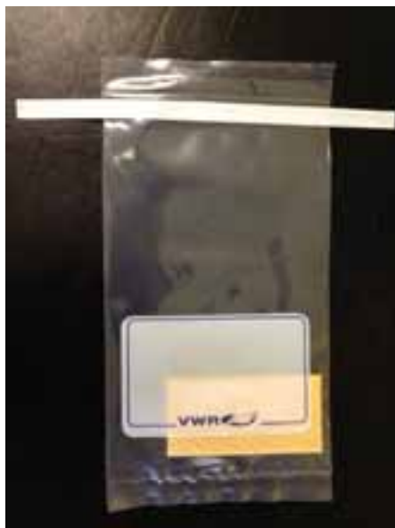
Figure 5. SANI-SPONGE, (Cat. No. 300-0230) sterile dry sponge in sterile bag used for sampling large surfaces.
