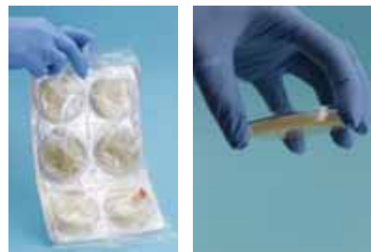
Figure 3. TSA contact plates (Cat. No. 271114ZI). The medium is pressed against the surface to take a sample of the environment. The special blister single packaging enables the use of a single plate at a time.
